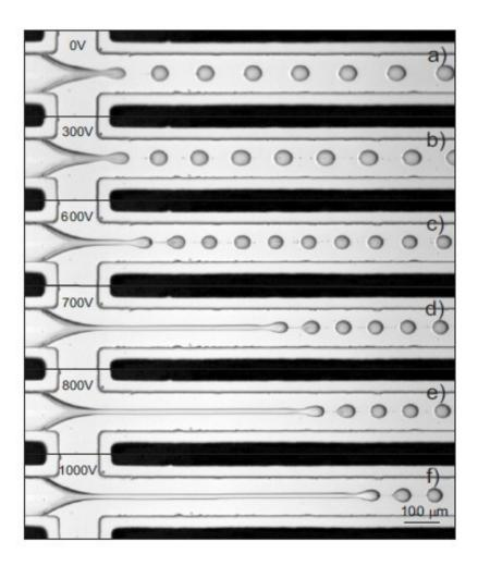
KCl 3 mS/m ; 9 kHz Inner flow rate: 50 μl/h Outer flow rate: 400 μl/h
