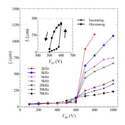
...and jet length depends strongly on frequency of the signal.
