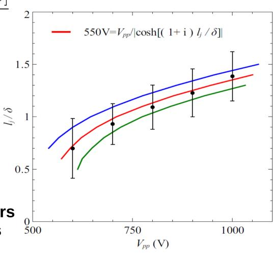
In all cases, jet breakup occurs when the voltage at the tip is around 550 V.
