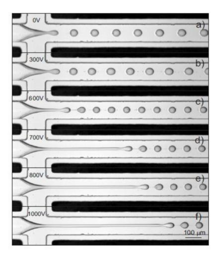
KCl 3 mS/m ; 9 kHz Inner flow rate: 50 μl/h Outer flow rate: 400 μl/h ...and jet length depends strongly on frequency of the signal.
